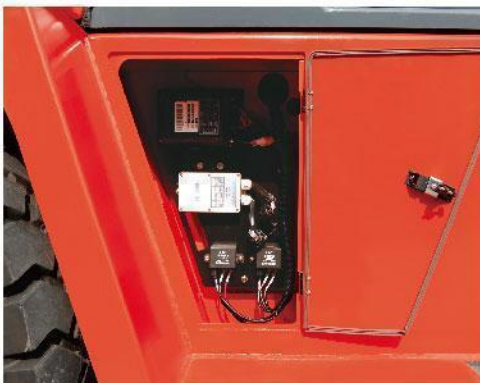
Independent integrated electric cabinet
